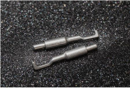
*L-tip part for a device used in endoscopic surgeries programmed with ESPRIT and machined on a Tsugami BO326.*
